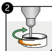
2 Operate in a clockwise direction. Maintain outward pressure.
